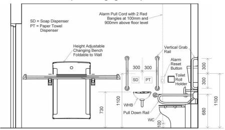
Figure 5 (Elevation) - Toilet for Assisted Users (with Changing Bench)
