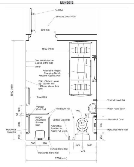
Figure 5 (Plan) - Toilet for Assisted Users (with Changing Bench)
