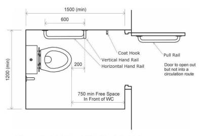
Figure 3 - Enlarged Disabled Cubicle
