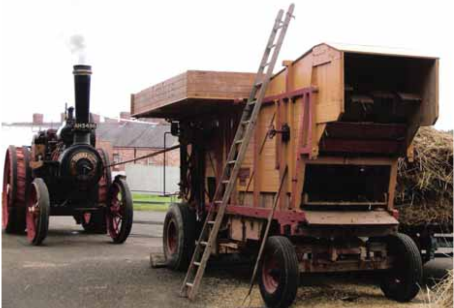
A portable threshing machine (Photo courtesy of Ulster Folk and Transport Museum)
