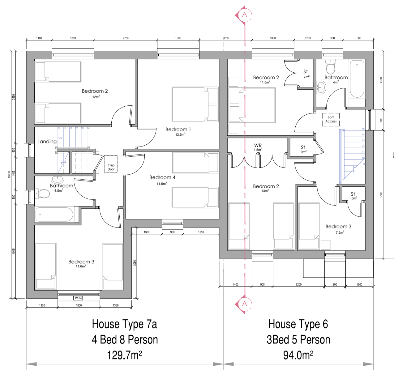
First Floor Plan. Scale 1:100 Total Floor Area HT6- 94m 2 Total Floor Area HT7a - 129.7m 2
