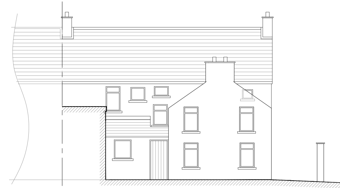
EXISTING REAR ELEVATION - SouthWest Scale: 1:100
