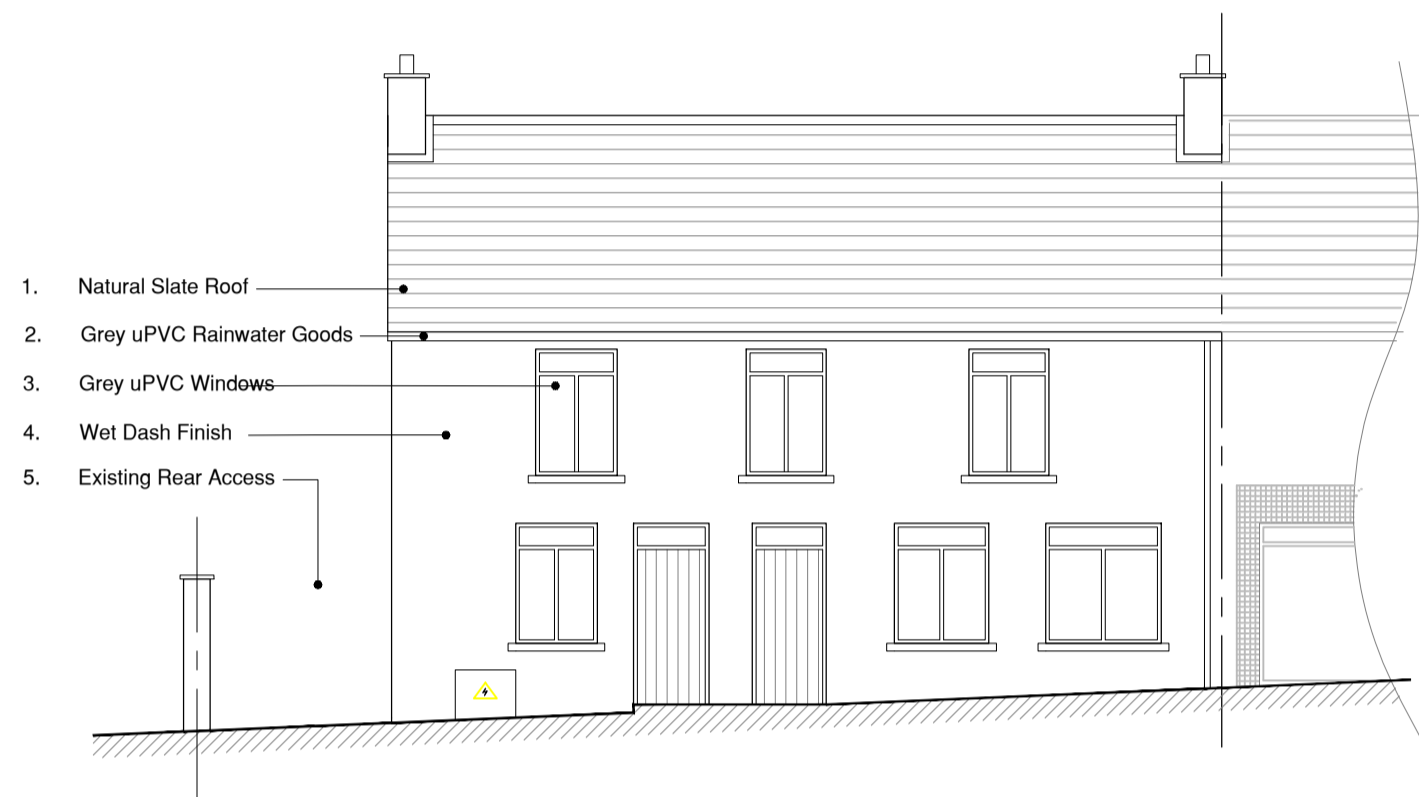
PROPOSED FRONT ELEVATION - NorthEast Scale: 1:100
