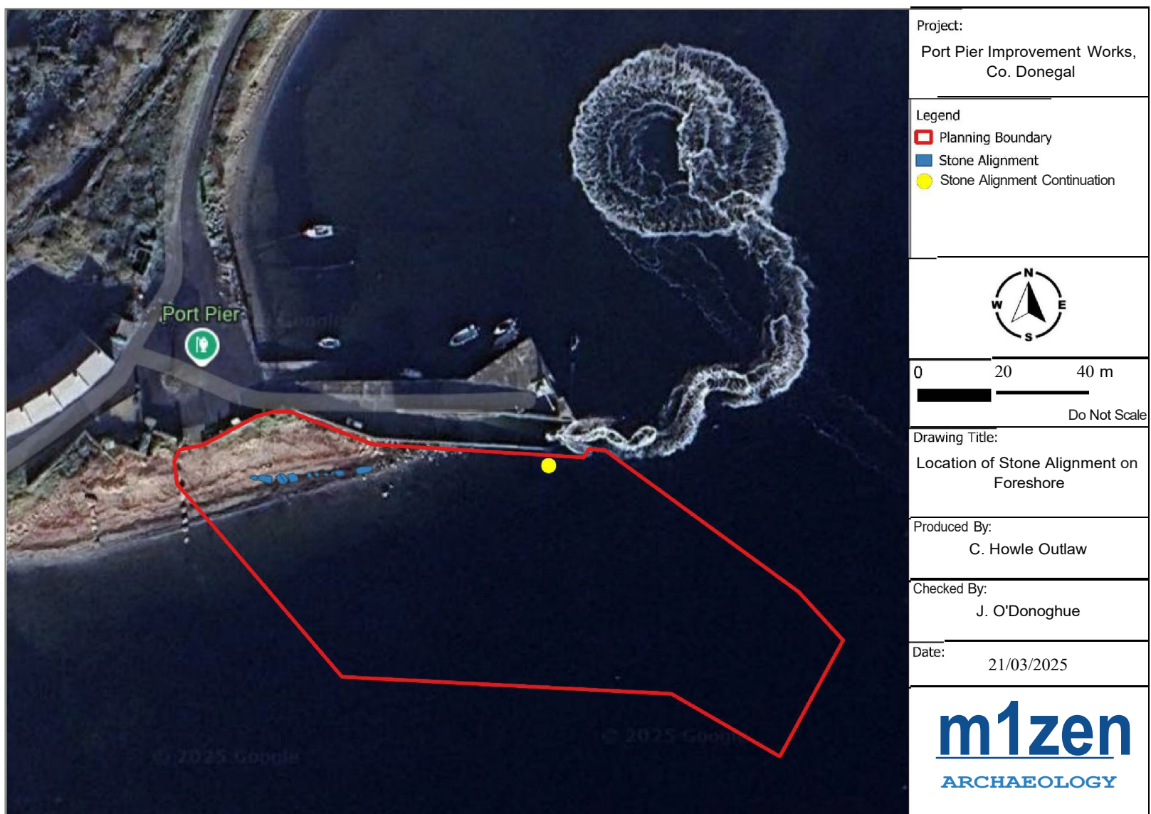
Figure 8: Locations of potential early piers/ slipway structure based on surveyed stone alignments.
